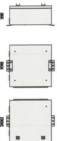
FIBER TELCO ENCLOSURE DETAIL
