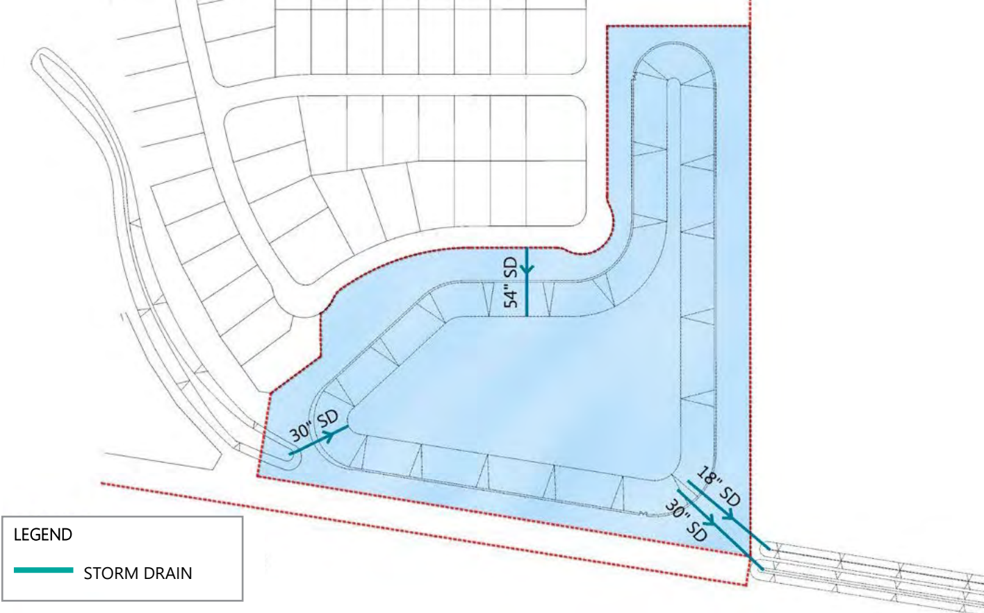
Figure 10.1.1A: Phase 1 Detention Basin
