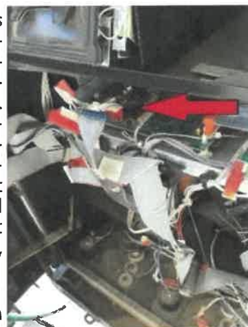
Card skimmer installed inside gas pump
